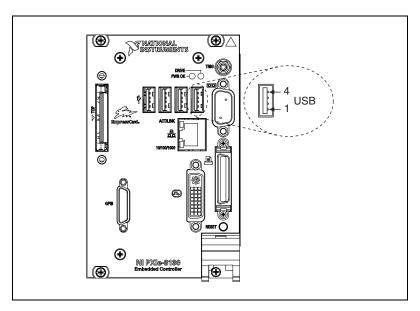
Figure 3-6. USB Connector Location and Pinout
